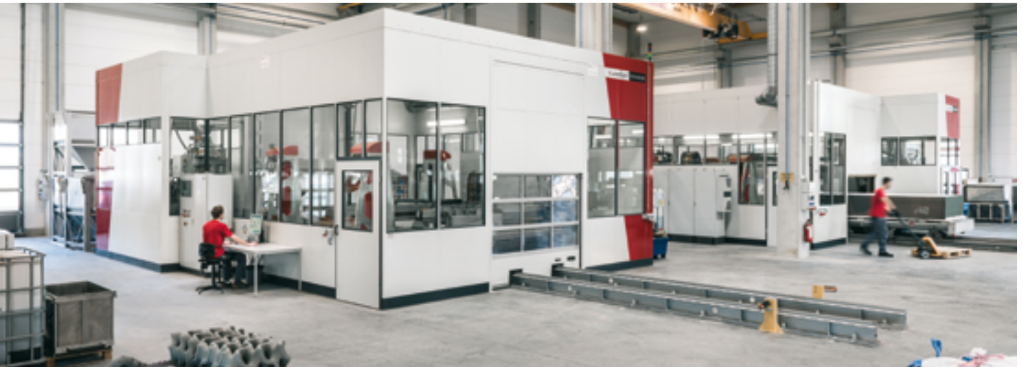
The largest 3D printer in the world has a print chamber measuring 4,000 x 2,000 x 1,000 millimeters (LxWxH). With its high-quality components, it is designed for continuous operation.
