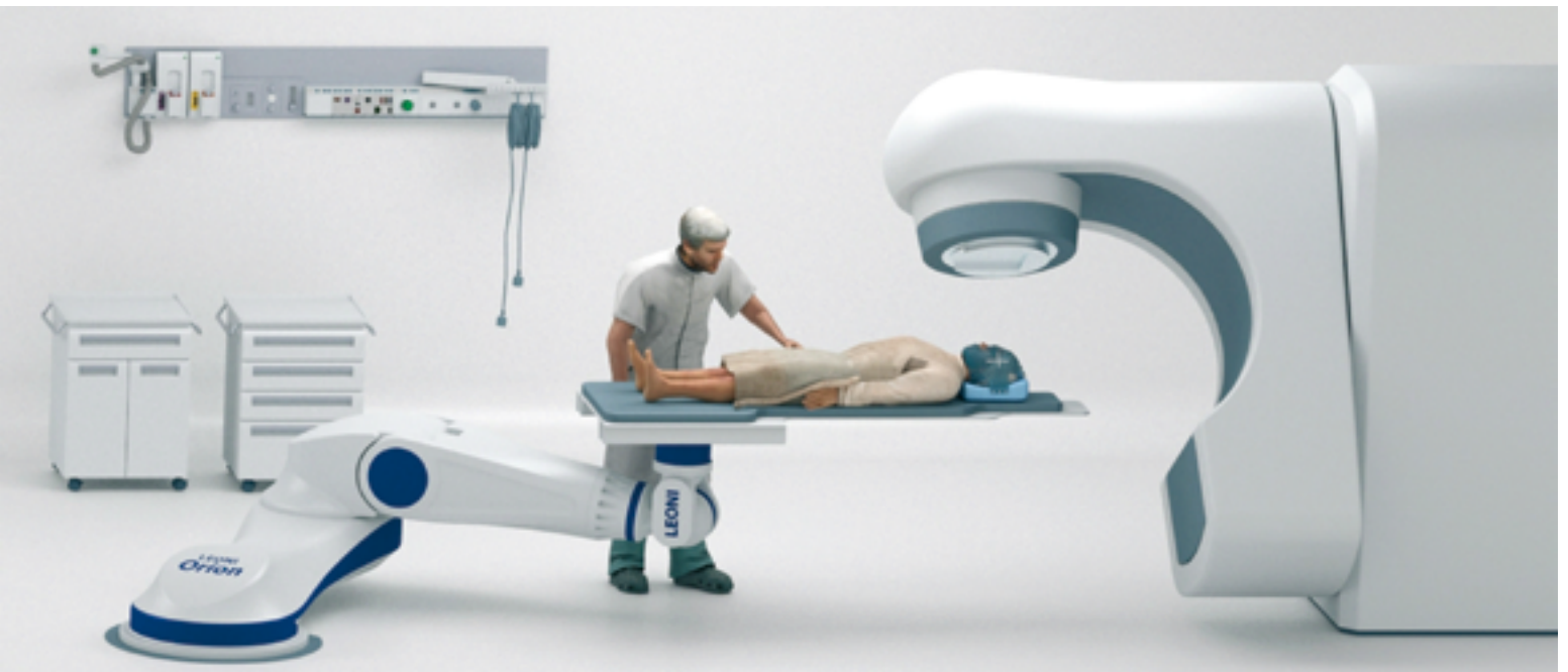
Working side-by-side with human nursing staff, LEONI ORION relies on B&R's SafeMOTION functions to meet the strict safety regulations for medical collaborative robotics.
