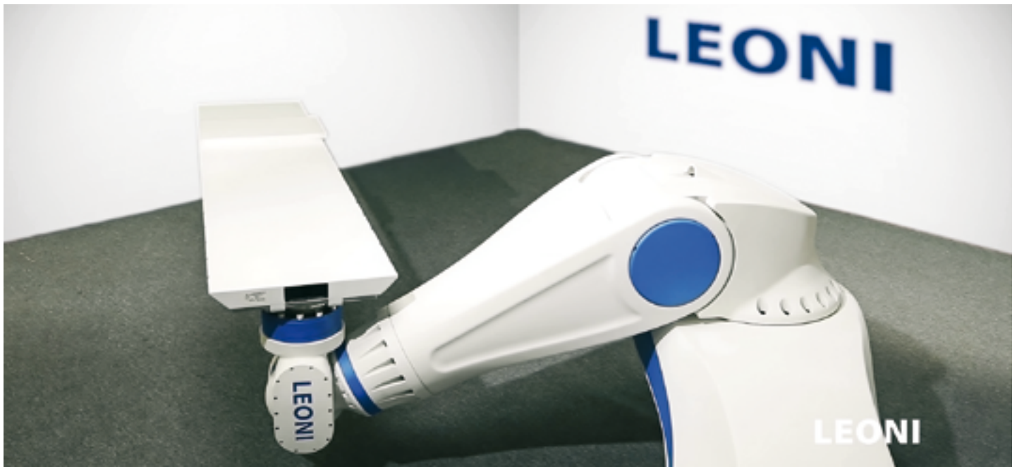
LEONI ORION offers dynamic positioning control with six degrees of freedom and sub-millimeter accuracy.
