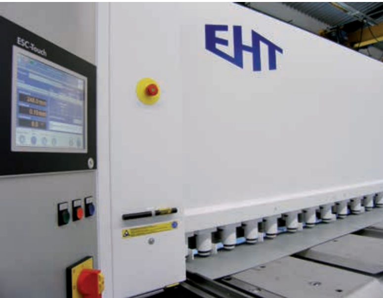
EHT's MultiCut series of power squaring shears, featuring an ECS touch screen controller, is designed for one-off and series production of parts of all sizes. Its extensive selection of sophisticated options make it especially efficient and ergonomic to use.
