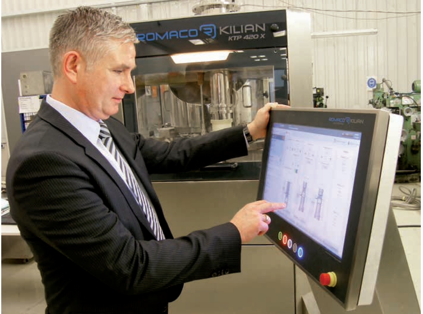
The newly designed HMI system with gesture control is based on a powerful Automation PC 910 with a dual-core i7 processor and a hygienic Automation Panel with a 21.5" display.
